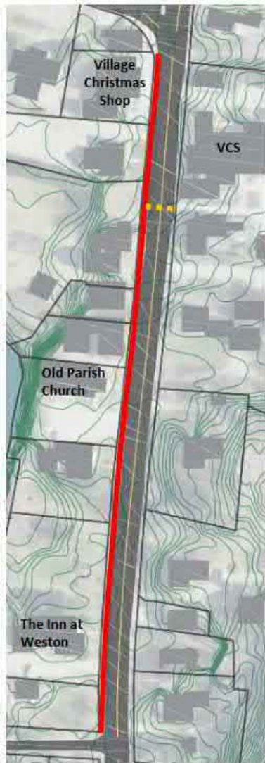
S1: Curbed sidewalk on west side of VT100, new crosswalk in vicinity of the Vermont Country Store.
