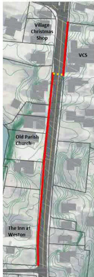
S3: Curbed sidewalk on west side from southern terminus to vicinity of VCS, new crosswalk at southern end of VCS, and extend sidewalk on east side headed north to Green.
